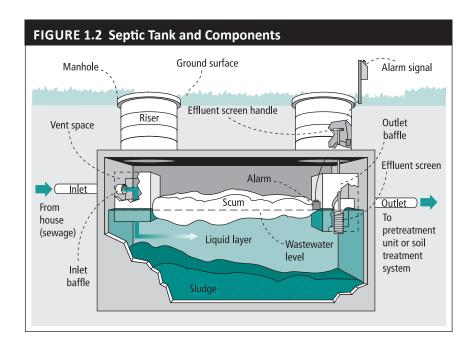
The size of the septic tank is based on the home's potential water use volume and the type of appliances used. In aerobic tank systems, pumps and other mechanisms are necessary to deliver air to the tank.
