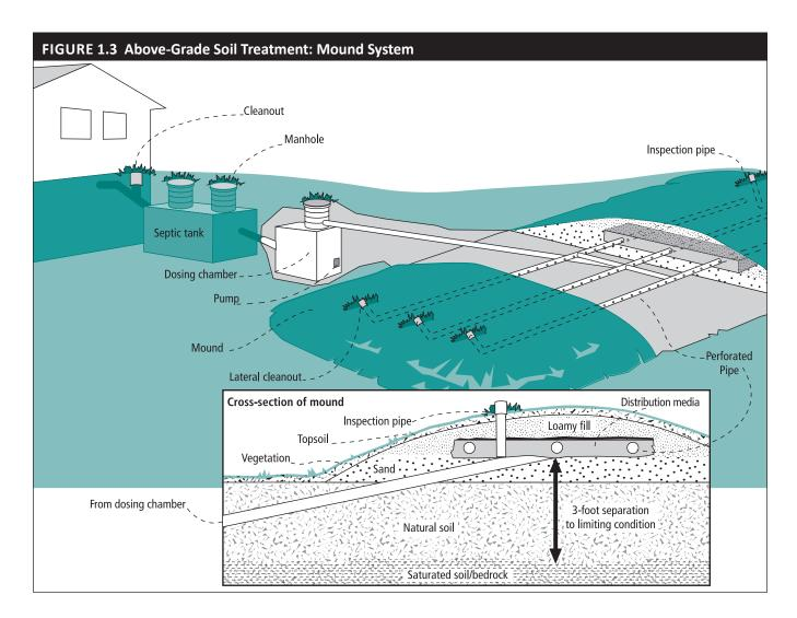
Pumps and a lift station may be components of a system where gravity flow is not possible. For example, in systems above grade and those using advanced technologies, a pump is required to provide pressurized flow for the distribution of effluent. Section 4 provides information about conducting legal and accurate site evaluations to determine the appropriate design for a given site.
