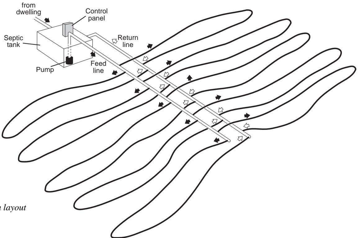
Figure 6. Drip system layout
