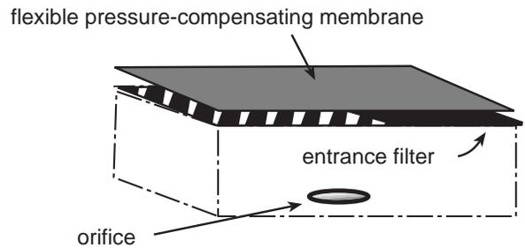
Figure 5. Pressure compensating drip emitter
