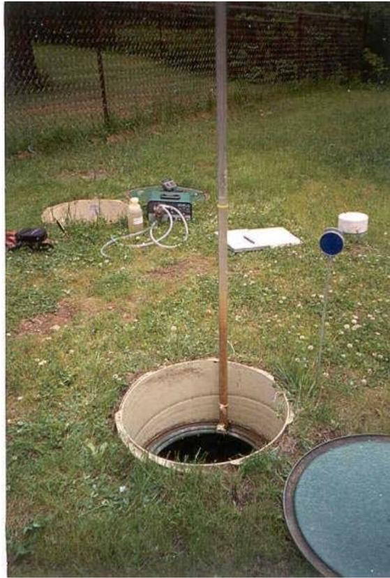
**Figure 6. Maintenance of sand filter systems is required to ensure that they are operating properly. This tube is being used to measure the scum and sludge depth in the septic tank. Some monitoring equipment is shown in the background.**
