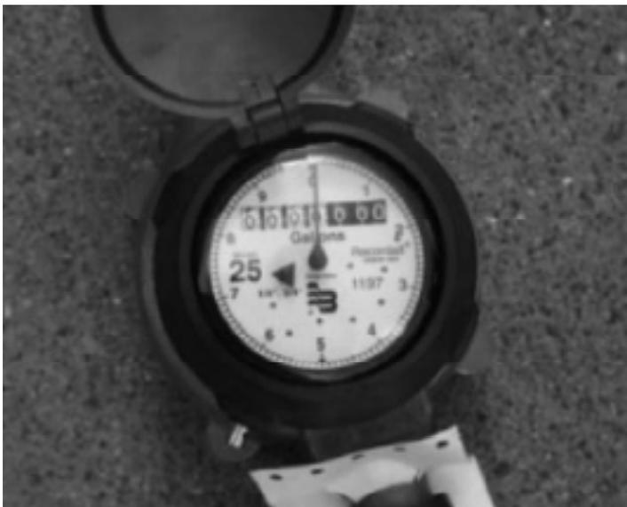
Figure 1. A typical water meter.
