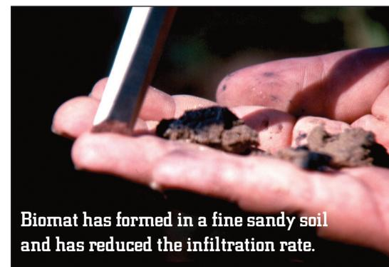
**Biomat has formed in a fine sandy soil and has reduced the infiltration rate.**
