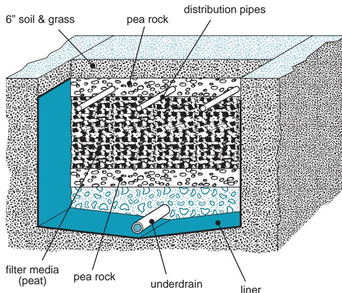
Figure 3. Lined peat filter cross section
