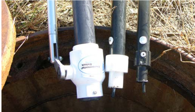
Figure 1. Sludge Measuring Instruments. (Left to right: Dipstick Pro, Sludge Judge II, Sludge Judge)
