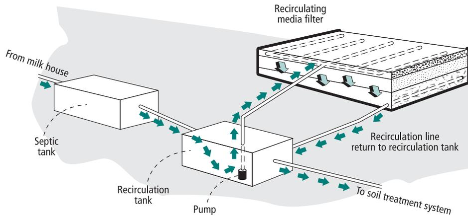
*Waste water flow path through recirculating media filter*
