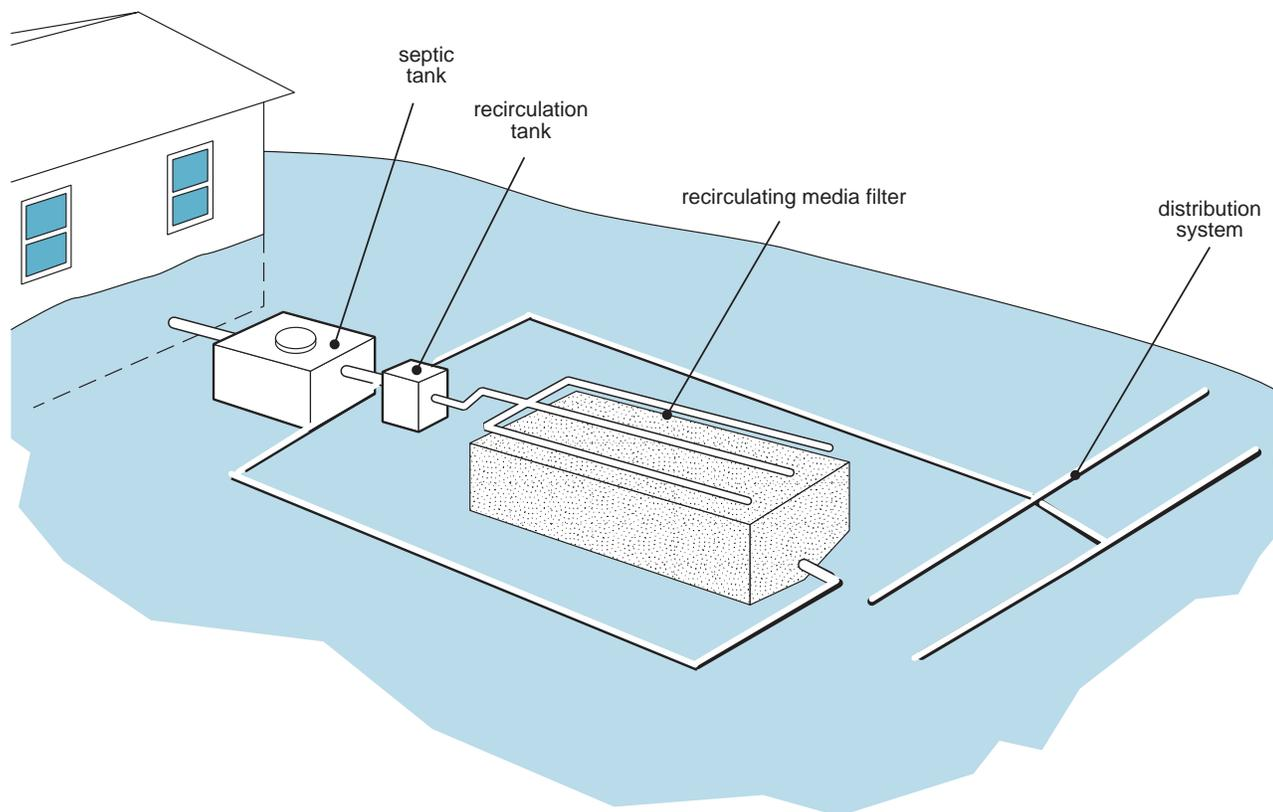
Figure 3. Recirculating filter system with pressurized trenches
