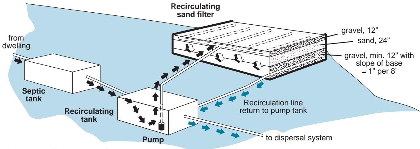
Figure 2. Recirculating media filter
