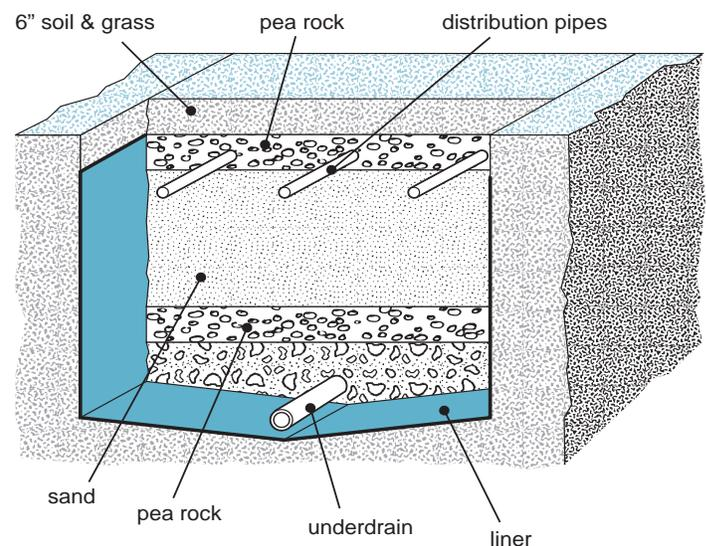
Figure 4. Low-rate (0.8–1.5 gpd/sq. ft.) sand filter
