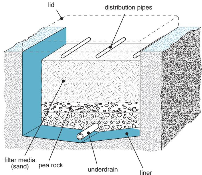
Figure 3. High-rate sand filter
