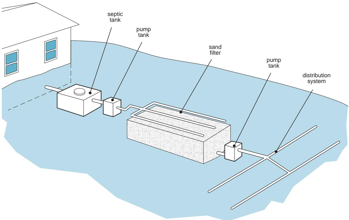
Figure 5. Sand filter system with pressurized trenches
