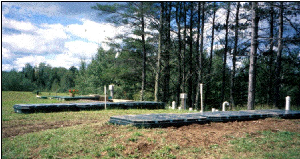
**Figure 6. Two sets of modular peat filters (each set sized for a 3-bedroom home) testing the Irish peat in one set of modules and a Minnesota peat in the other modules.**
