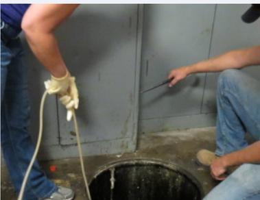
At truck facilities connected to city sewers, researchers took wastewater samples from flammable waste traps while trucks were washed.
