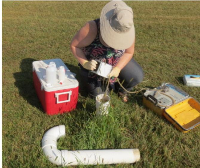
A researcher collects a nonwinter wastewater sample from the holding tank at the Shakopee facility.
